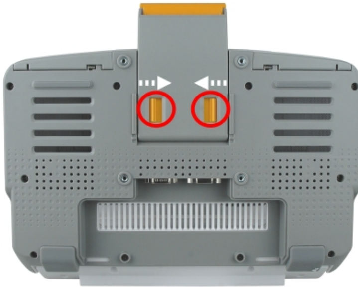
Figure 3-9: Release the Stand
