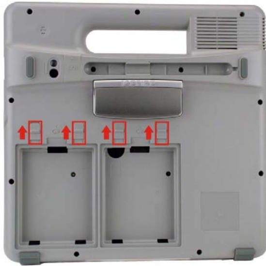
Figure 3-1: Release Battery Latches
