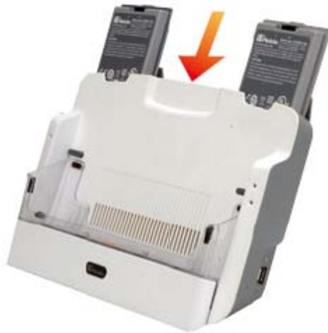
Figure 3-6: Insert Batteries to Docking Station
