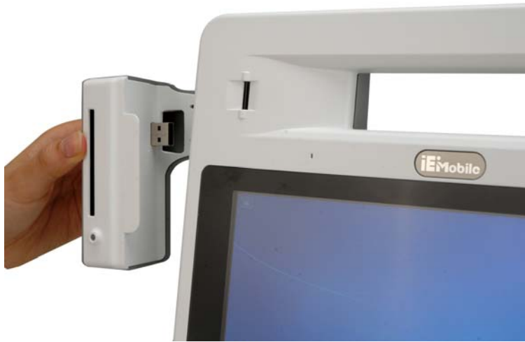
Figure 3-15: Smart Card Reader Installation
