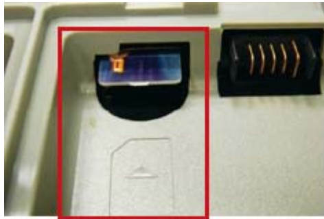
Figure 3-8: SIM Card Installation
