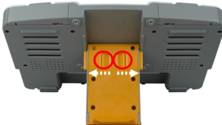
Figure 3-10: Lock the Stand
