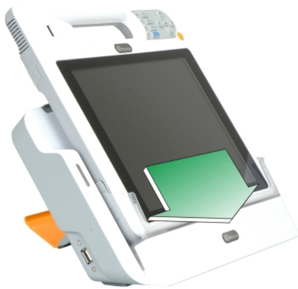
Figure 3-11: Place the ICEFIRE-T10A to the Docking Station
