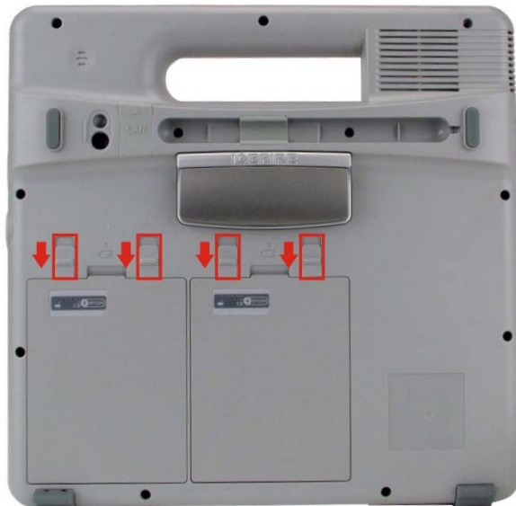
Figure 3-3: Lock the Battery
